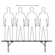
In the FE analysis, the previous underframe was compared with the new underframe. The table or bench legs were clamped tightly for this purpose at the top and at the snapper. A force F acts from the outside at the bottom. This calculation method simulates swaying in the longitudinal direction.
